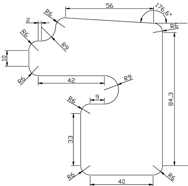
Fig. 26. Test pocket (all dimensions are in mm).
