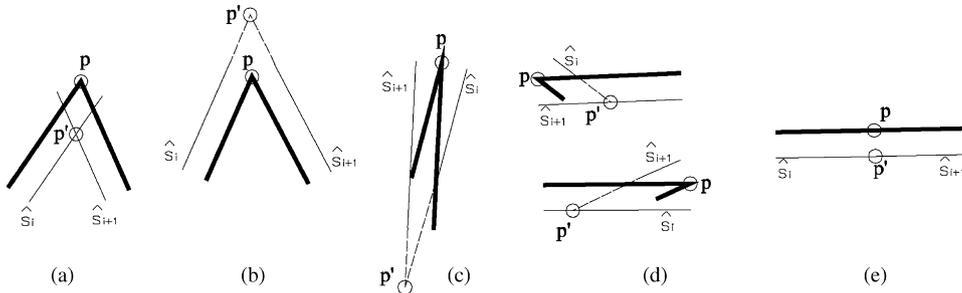
Fig. 6. The combination between two line segments and some cases of the types of the base intersection point  $p'$  for  $\hat{s}_i$  and  $\hat{s}_{i+1}$ : (a and e) a TIP for both  $\hat{s}_i$  and  $\hat{s}_{i+1}$ ; (b) a PFIP for  $\hat{s}_i$  and an IFIP for  $\hat{s}_{i+1}$ ; (c) an FFIP for  $\hat{s}_i$  and an IFIP for  $\hat{s}_{i+1}$ ; (d) an IFIP for  $\hat{s}_i(\hat{s}_{i+1})$  and a TIP for  $\hat{s}_{i+1}(\hat{s}_i)$ .
