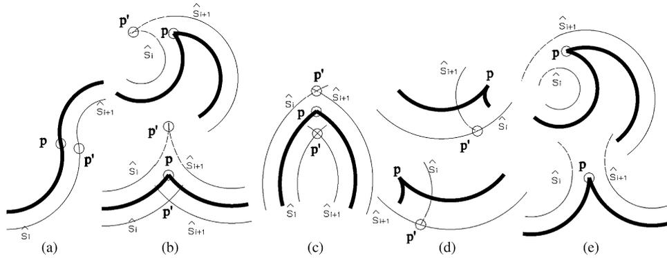
Fig. 10. The combination between two arcs and some cases of the types of the base intersection point  $p'$  for  $\hat{s}_i$  and  $\hat{s}_{i+1}$ : (a and b) a TIP for both  $\hat{s}_i$  and  $\hat{s}_{i+1}$ ; (b and c) a PFIP for  $\hat{s}_i$  and an FIP for  $\hat{s}_{i+1}$ ; (d) an FFIP for  $\hat{s}_i$  and an FIP for  $\hat{s}_{i+1}$ . (e) There is no base intersection point between  $\hat{s}_i$  and  $\hat{s}_{i+1}$ .
